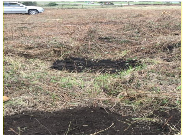
Photo 12. Surface scrapes taken surrounding TP7 to delineate the extent of the waste
